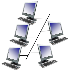
shared wire (e.g., cabled Ethernet)
